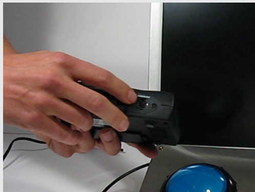
A simple 8 pin connector on the media player provides an interface for buttons >
