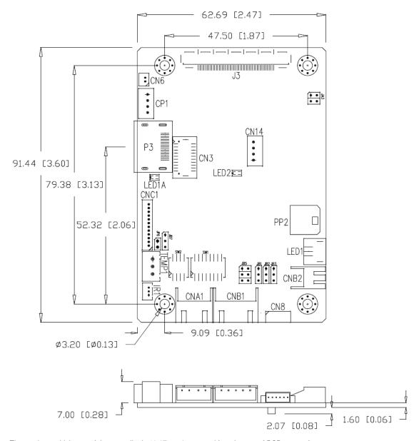
The maximum thickness of the controller is 10.67mm (measured from bottom of PCB to top of components, including any underside components & leads). We recommend clearances of:
