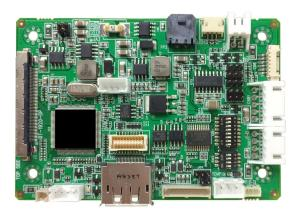
The Digital View DT-1920-DP LCD controller board with single Displayport input and LVDS panel connection support for general commercial and industrial applications. Compact and highly reliable this controller board incorporates advanced features such as Digital View's multi panel timing support, brightness & temperature sensors, auto-EDID setting and audio line out
